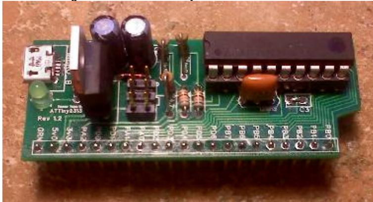
In the figure above, we have the USB connector on the left, a green LED and resistor to indicate that we have power from the USB connector, the 6 pin programming header, two diodes, the voltage regulator and its two capacitors, five resistors, a 12-Mhz resonator, and the ATTiny2312 micro-controller that does all the work. Then at the bottom of the PCB there are 21 pins that allow us to place these into a breadboard allowing us to build USB devices.
