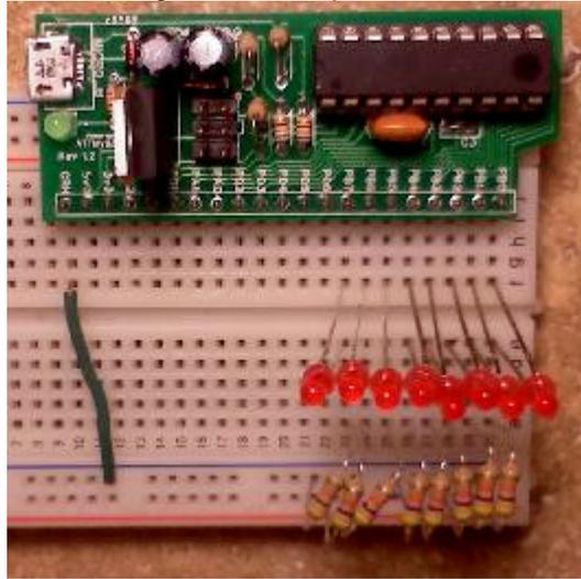
Connect the programmer to the Host and the breakout board.
