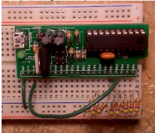
Once you have connected the device to the host, send the request in Table Q-3. You should get an 8-byte array of all zeros. Now, take the long lead wire and connect the breakout board's 3v3 pin to PB4 on the breadboard, as shown in the figure above, and request the packet again. You should now get an array of seven zeros and a one. Try connecting the lead to other pins and requesting the packet again.
